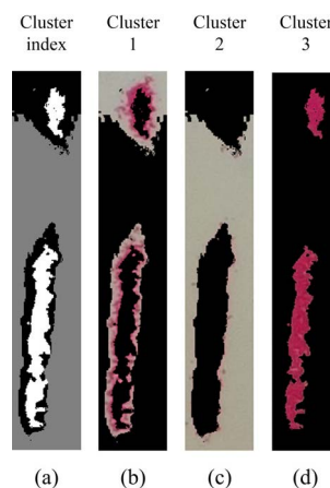
FIGURE 8. A sample of a) cluster index, (b) cluster 1 represent background 1, (c) cluster 2 represent background 2, and (d) cluster 3 represent foreground.
